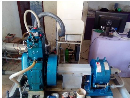
Kirloskar TV1 Engine experimental setup.
